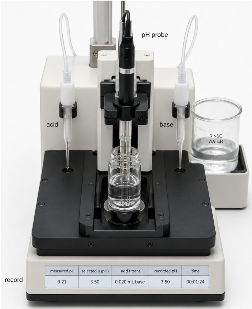
Figure 2: Robotic pH-conditioning station.
